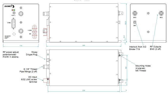
Heatsink in contact with coolant water. Default aluminium. See BR option. Water-coolant fittings supplied are suitable for 8mm OD / 6mm ID pipe.
